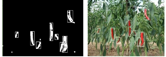
Figure. 15. Example of Blob Analysis output for Data 2
